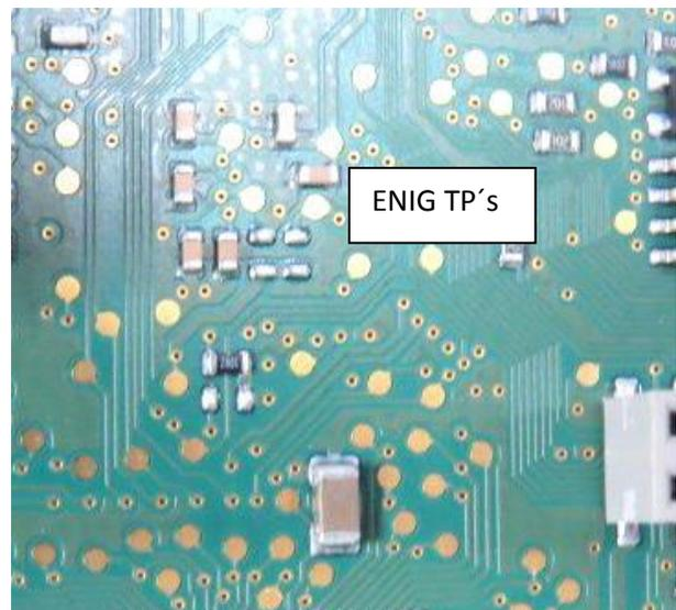
If the PCB has a lot of TP's, it can be a challenge to make sure the printboard does not bend a little when testing. It will not be a problem if it is not ENIG, but we have to take some precautions when designing the fixture.
